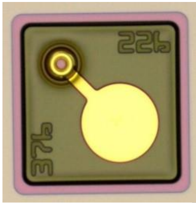
A TYPICAL WAFER PROBER TESTED VCSEL
